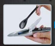
1 Apply 1-2 drops onto the prism.
